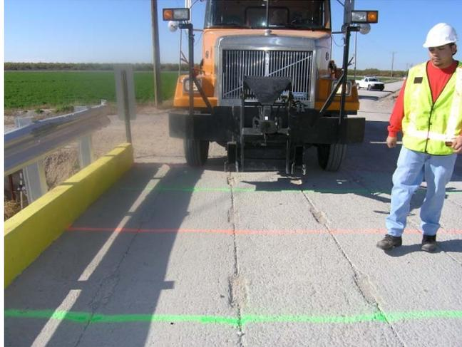
**FIGURE 1 Load Rating Prestressed Concrete T-Beam Bridge by Proof Testing**
